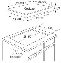
\*Depth of unit at conduit location (right rear) is 4-5/8"
